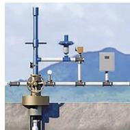
Plunger Lift is one of the most economical ways to achieve maximum deliquification, particularly in marginal and aging wells. Plunger lift uses the well's own energy in combination with a plunger—that functions like a swab—to lift and remove accumulated liquids
